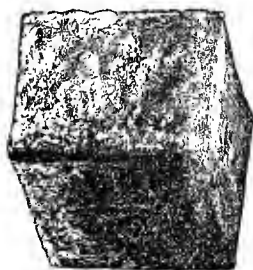
FIG. 87.—FRACTURE AT LOW TEMPERATURE.†
